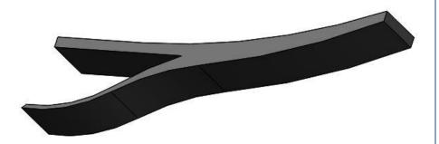
**The Molded Foot** is made of strong rubber that flexes but maintains its shape. This piece is fixed to the bottom of the ankle joint and it contact the ground upon impact. The foot moves with the ankle joint, which is controlled by the pneumatic piston.
