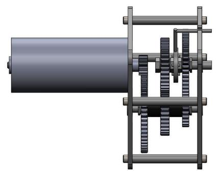
distribute forces without intersecting with gear motion. A selector gear is used to engage with one of the two gears on the output shaft.
