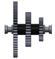
The output shaft (shown right, below) contains the two final stage gears that interface with the input shaft. These spin freely on the output shaft until they are engaged. When the selector gear engages with one of the gears, the nubs match up with the holes on the gears themselves to robustly transfer motion to the output shaft.
