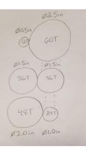
Ft-Fn+Fs=0 36t - Ft (2.5/2in) + Fs (0.5in)=0  $F_{s} = 37.51b(1.25in)/(0.5in)$ = 93.75 15 on 36T Final M.= (1.5/2in)93.75 = 70.31 in 16 Fs= 70.31 in 16/2.0 in = 35.1616 on 48T Final Sn
