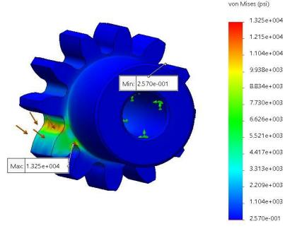
**This 12T gear** (shown above) is part of the planetary gearbox system. The forces acting on it represent the force interactions between the central 48T motor gear and each of the corresponding planet gears. These stress values seem to be within reasonable tolerances given the application of the gears in transmitting torque and motion.
