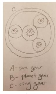
ratios. The final gearing choices produced output ratios of 1:5 and 1:10 reductions.
