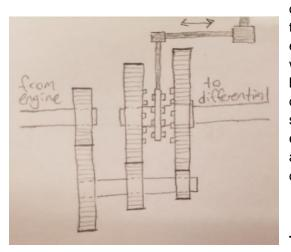
determine the position of the gears relative to each other and mark out what parts would need to be created. The general design involved an input shaft from the motor or engine, a lay shaft, and an output shaft to the differential.
