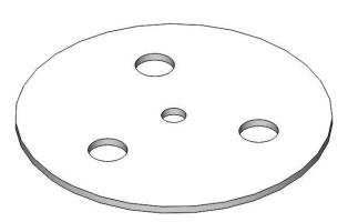
both ends with bearings. This includes three holes for press fit of these bearings as well as a middle clearance hole for the motor shaft.
